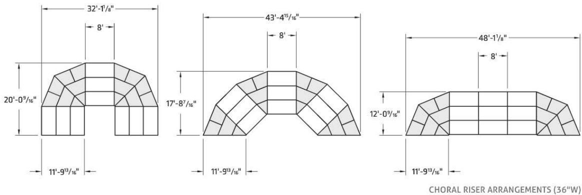
STRAIGHT RISER AND PIE SECTIONS MAY BE USED TO CONSTRUCT A VARIETY OF ARRANGEMENTS
